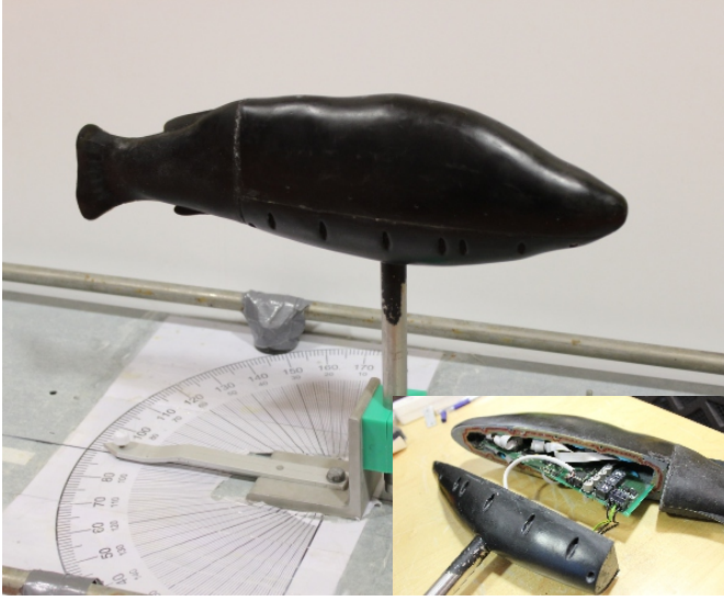
Figure 2: The artificial lateral line probe: the closeup image (bottom left) shows the open electronics bay, the cables are fed through the stainless steel mounting pole. Location of the 11 lateral line piezoresistive pressure sensors (top right) and the set-up used in the experiments.
