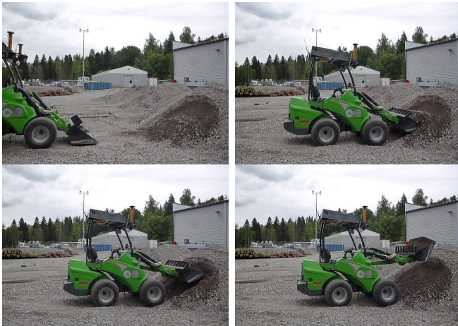
Fig. 5: Scooping sequence with Neural Network controller.
