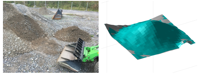
Fig. 10: Pile-transfer test for bucket filling controller evaluation: (left) workspace with scooping area at left and dump pile at right; (right) surface model of dump pile after one job, used to estimate volume.
