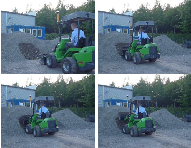
Fig. 2: Manually driven scooping action for data collection.
