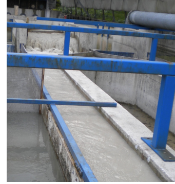
Fig. 6. Flume used for semi-natural-environment experiments.
