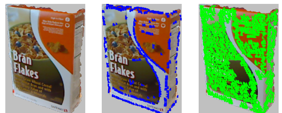
Fig. 2. Visualization of different ECV features. Left: Input RGB-D model. Middle: ECV segments in blue. Right: ECV texlets in green.
