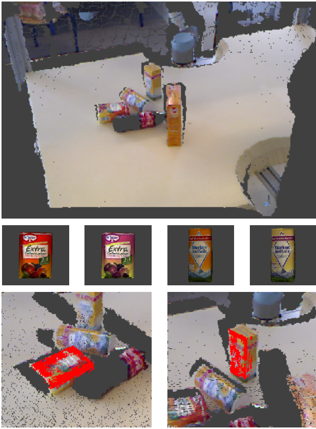
Fig. 7. Pose estimation results from our setup. Top: input Kinect scene. Middle: input textured KIT objects (leftmost instances) and their color calibrated versions (rightmost instances). Bottom: estimation results for both objects, aligned objects overlaid in red.
