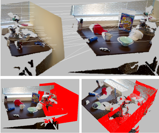
Fig. 6. Registration of two different views of the same scene using our optimized RANSAC algorithm. Top: input Kinect views, showing 25 randomly selected correspondences computed using ECV context descriptors. Bottom left: registration result with the aligned version of the leftmost scene view in the top image overlaid in red. Bottom right: zoom of the aligned point sets. Note the high quality of the alignment, which is performed without refinement.
