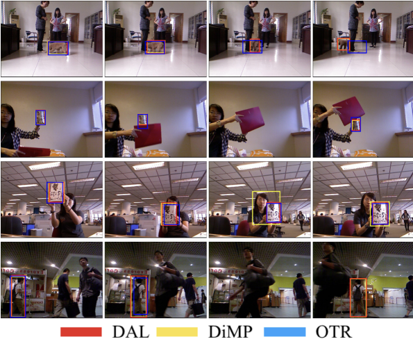
Fig. 3. Qualitative comparison of DAL, OTR [5] and DiMP [7] on the PTB. All trackers localizes the target and give precise bounding boxes (the first two rows). DAL shows better discriminative ability when strong distractor appears (human face in the third row). DAL reports target disappearance more accurately. Song would like to add the OTR results
