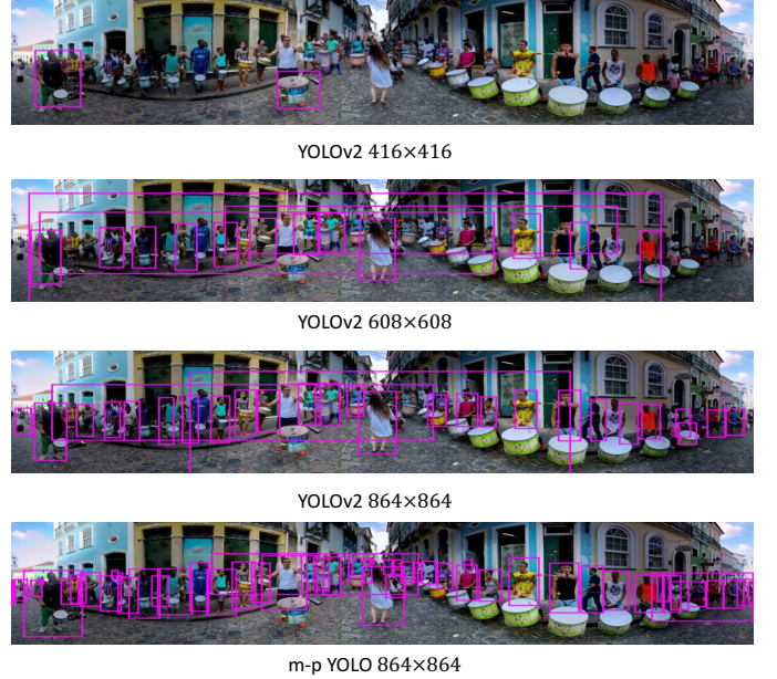
Figure 10. Examples of human detections with different resolutions and with multi-projection YOLO. Best viewed on display.
