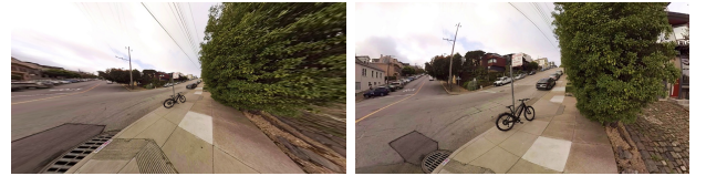
Figure 7. Perspective (left) and stereographic (right) projections of the same spherical image. The FOV for perspective projection is set as h = 90^\circ , w = 175^\circ ; The FOV for stereoprojection is set as h = 90^\circ , w = 180^\circ . For wide-angle projection, stereographic model preserves better information although straight lines are not preserved.
