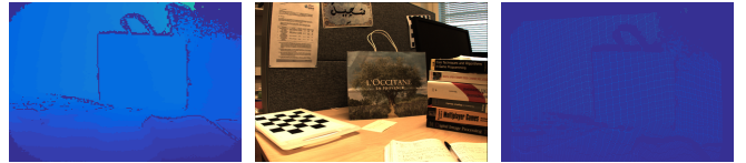
Fig. 1: Highly sparse depth maps. From left to right: original depth map, RGB image and warped sparse depth map.
