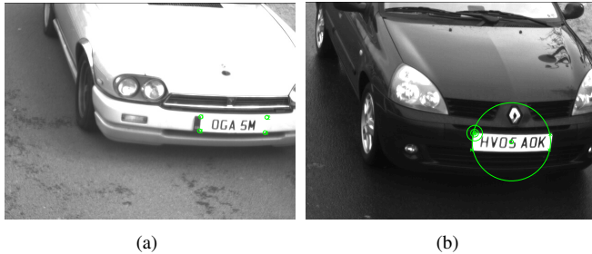
Fig. 15. License plate database: (a) Example image where corners marked with green circles (b) Demonstration of accuracy measure for license plate localisation (green circles in the upper left corner).
