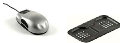
Figure 3.8.1: VTPlayer tactile mouse
