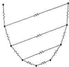
Figure 4: Heart wall modelled by spring elements.
