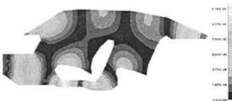
Figure 13: Velocity in car enclosure (x direction/amplitude) at 350Hz by initial mesh
