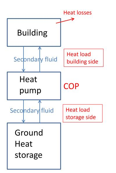
Design of the storage configuration must ensure high performance for the heat pump during operation
