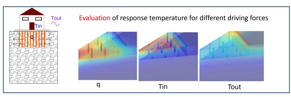
The response temperatures in points of interest is extracted (Borehole surfaces)
