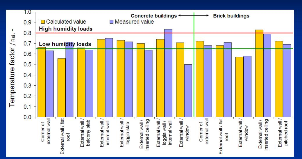
92% of the temperature factors  $f_{Rsi}$ <0.8 ( $\Delta v \sim 6 \text{ g/m}^3$ )
