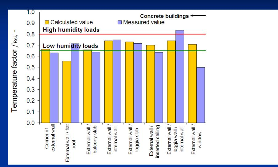
92% of the temperature factors  $f_{Rsi}$ <0.8 ( $\Delta v \sim 6 \text{ g/m}^3$ )
