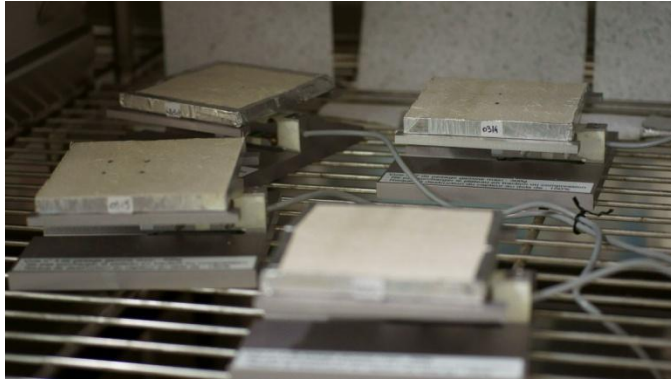
Samples of dimensions 100x100x10 mm, insulated on 5 faces
