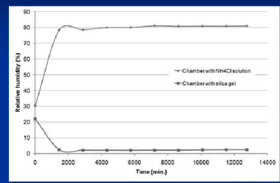
We can see that the distribution of relative humidity in the separated chambers simulated by specific saturated salt solutions was after certain time from the experiment beginning (typically after 16 hours) relatively well constant. This is very important finding, because it validates the proper conditions of the experiment.
