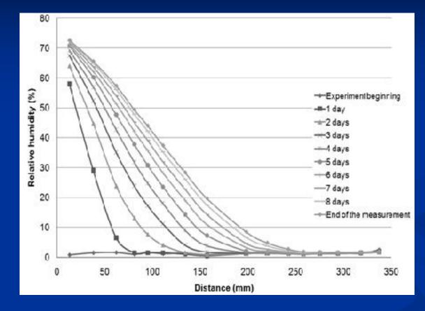
In figure, there are presented relative humidity fields measured within the transient experiment. We can see relative humidity distribution along the sample length caused by difference conditions of simulated environments.
