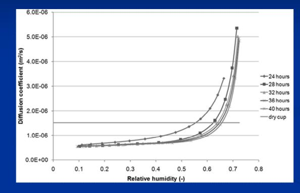
there are presented results of water vapour diffusion coefficient and resistance factor calculated using inverse analysis of measured relative humidity fields. Here, the data accessed using standard dry cup method is given as well.
