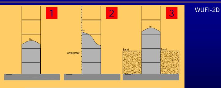
Configuration 2 was one side completely covered with tiles. Configuration 3 had saturated sand to a height of 45 cm. The sand was saturated (100% RH) during the tests.
