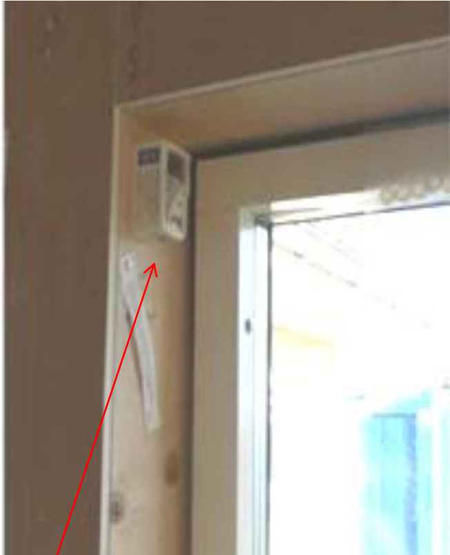
Loggers were placed inside of the wall on the stud
