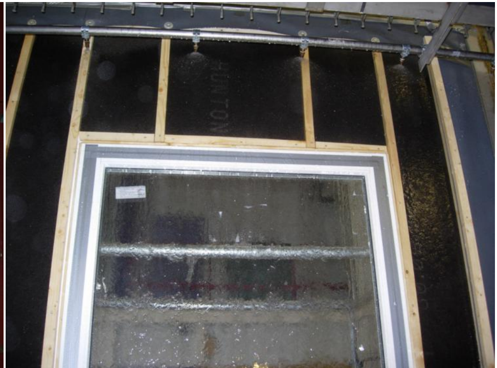
Inside the test chamber, nozzles spraying water on the test section
