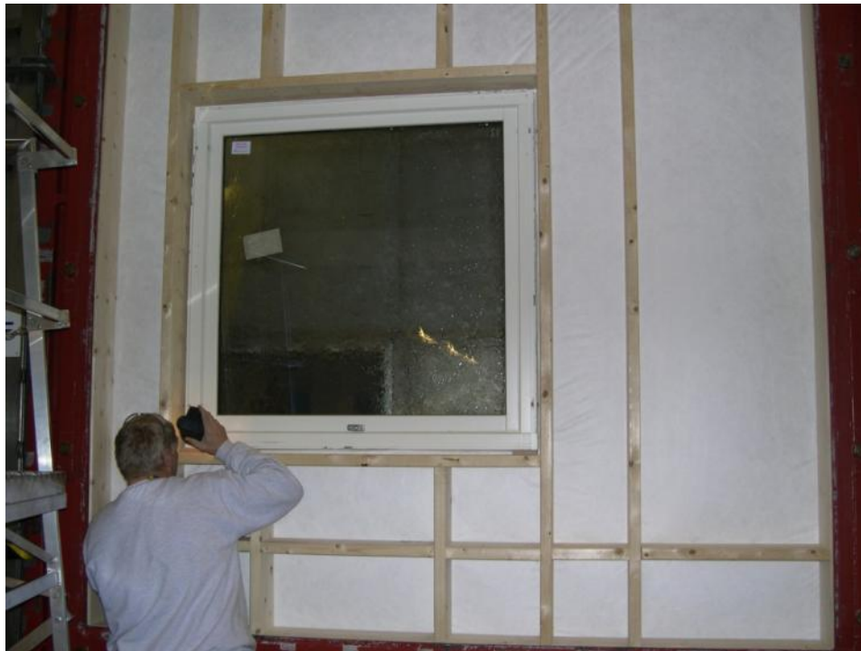
Test chamber visual observation of water leakages
