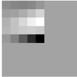
Figure 1.8: Non-symmetric LPA masks for estimation (smoothing) and differentiation. The LPA window weight w is Gaussian, the first quadrant. The reference pixel is at the right down corner of mask depicted into the larger extended mask (grey square 11 \times 11 ). The grey color corresponds to zero values of the mask values. The LPA power m = 1 . The estimation mask size is 5 \times 5 , h = 5 . Black and white define a scale between smaller and larger values of the kernel values.
