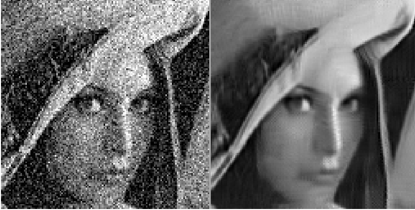
FIG. 4.4. Lena phase images: noisy phase observation (left) and iterative CDBM3D phase reconstruction (right), \sigma = 0.3 . PSNR for the reconstruction is 40.29 dB and for the noisy phase is 29.27 dB.
