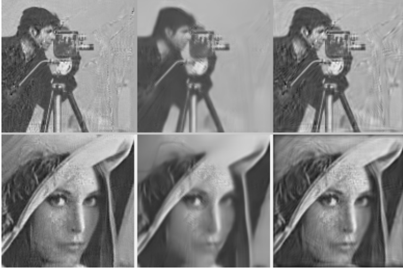
FIG. 4.6. Reconstruction of varying phase (cameraman) and amplitude (Lena): from left-to-right: BM_2 , Sp , WFT algorithms, noisy observations, \sigma = 0.1 .
