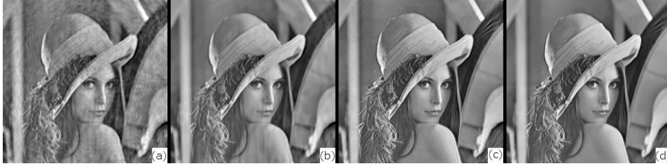
FIGURE 5. The filtering effects in the phase reconstruction by the MF-DDT algorithm ( z_j=1.5 \cdot z_f ): (a) L=1 , PSNR=15.9 dB (no filtering); (b) L=1 , PSNR=16.4 dB (with filtering); (c) L=10 , PSNR=16.8 dB (no filtering); (d) L=10 , PSNR=17 dB (with filtering).
