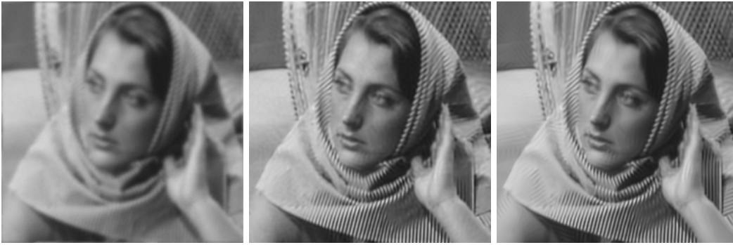
Fig. 1. Examples of image deblurring (Image 'Barbara' 256x256, From left to right: blurred image, Gaussian blur (kernel 25x25, std = 1.6); noise added variance 2; deblurring by GSR , PSNR = 28.6 dB, deblurring by our method, PSNR = 28.8 dB)
