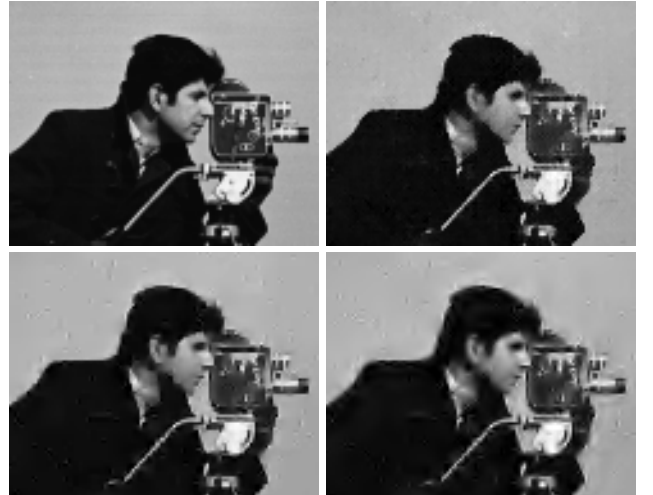
Figure 7: Denoising of the Cameraman image, \sigma = 25 . Clockwise from top-left: original image, anisotropic LPA-ICI estimate, PSNR=28.1dB, translation-invariant Daubechies wavelets (DB4), PSNR=27.4dB, and translation-invariant Haar wavelets, PSNR=27.8dB.
