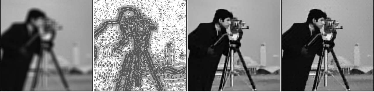
Figure 1: Cameraman image, from left to right: blurred noisy observation (9x9 box-car PSF, Poissonian noise \chi=17600 ), adaptive block-sizes (dark gray h_{j+}=4 , white h_{j+}=16 ), deblurred estimate \hat{y}^{\text{RWI}} ( ISNR 6.63dB), and Poissonian Anisotropic LPA-ICI RW estimate ( ISNR 6.55dB).
