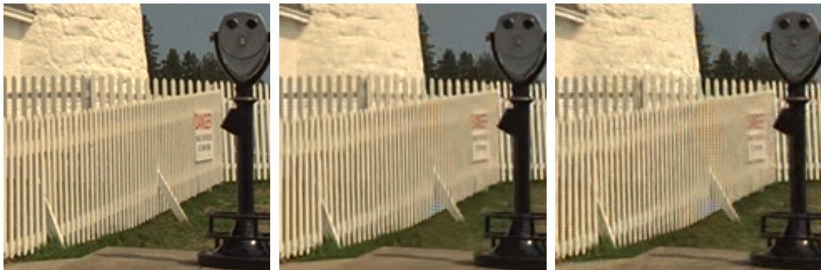
Figure 5. From left to right: ground truth, proposed denoising + interpolation [13], denoising [12] + interpolation [13]. Signal dependent noise ( a = 0.004, b = 0.02^2 ).
