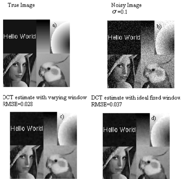
Figure 7. True “Montage” image; noisy image; the estimate with the varying adaptive window size ( \Gamma = 2.0 ); the estimate with the fixed ideal size window.
