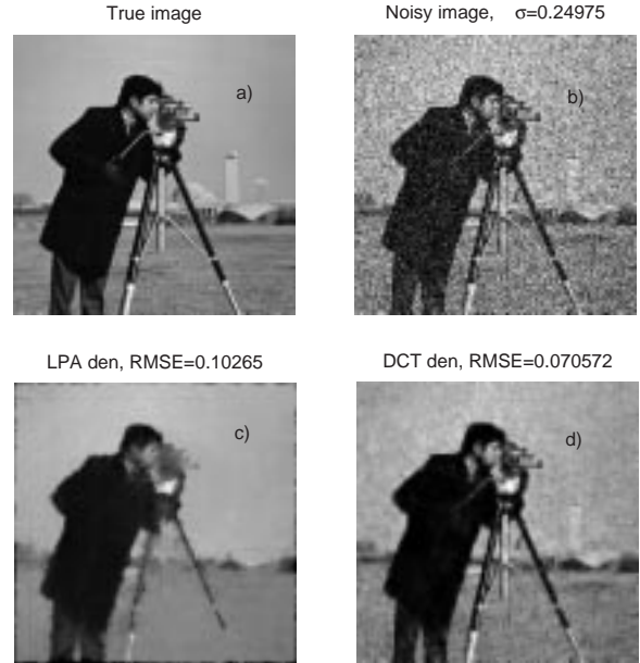
Figure 5. a) True image, b) Noisy image, c) LPA denoising, d) DCT denoising with ICI adaptive window sizes.
