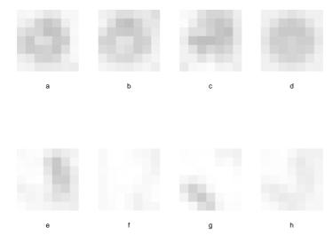
Fig.~5 Examples of dots in Heliotest images: (a)-(c) Regular dots; (d) Regular dot expectation; (e)-(g) Missing dots; (h) Missing dot expectation (note that the dot is not completely missing).
